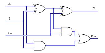
A and B are the input bits, and  $C_{IN}$  is the carry bit from a previous addition. S is the one-bit sum, and  $C_{OUT}$  the carry resulting from the addition.  $C_{OUT}$  is the  $C_{In}$  for the next full adder. The following table shows what the values are:
