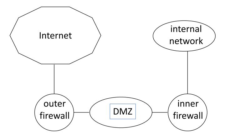
Two firewalls, one (outer firewall) connected to the Internet, the other (inner firewall) connected to internal network, and the DMZ is between the firewalls
